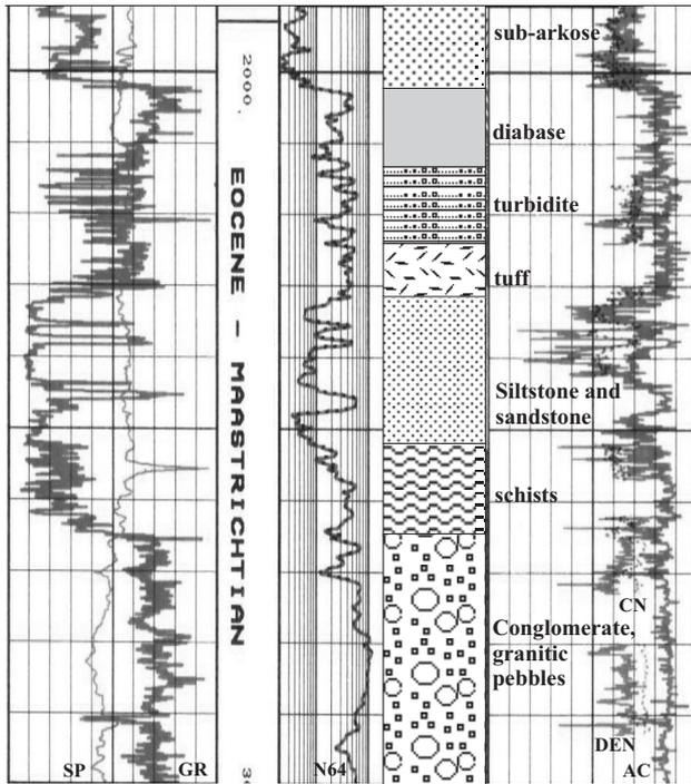
Fig. 6. Completion log of Cerna-1 well, interval 1900–3200 m.
