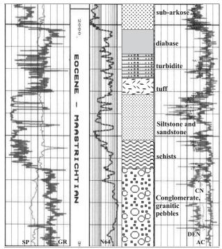
Fig. 6. Completion log of Cerna-1 well, interval 1900-3200 m.
