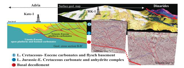
**Fig. 9.** Geological display showing position of 2D Seismic line "c" accros the part of the imbricate Adria carbonate platform. For the locations see Fig. 1. Published with permission INA-Naftaplin.
