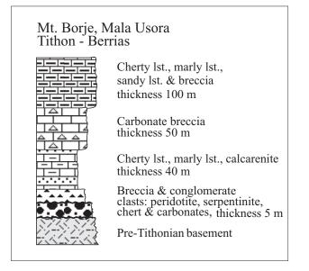
**Fig. 11.** Basal part of the Late Jurassic-Cretaceous foredeep overstep sequences in front of the Eastern thrust belt, Central Bosnia.
